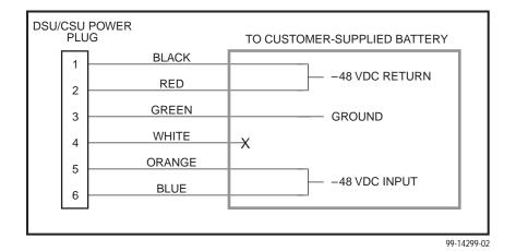
Figure 2-10. -48 Vdc Single Source Power Supply Pinouts
